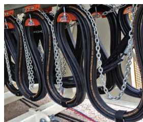
In vibrating applications, Grip Straps remain stationary while allowing proper hose expansion.
