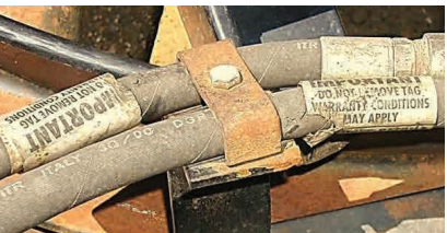
Traditional fixed hardware can cause catastrophic damage to hoses. Python Straps allow natural hose expansion & contraction.
