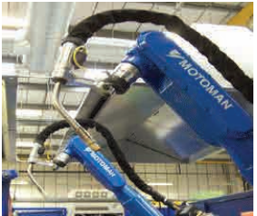
Weld Shield protects expensive hoses on large robotic welders.
