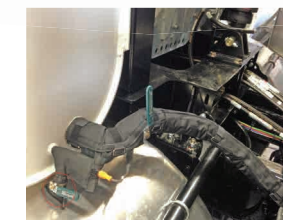
Radiant Lined 1050 is tailored to insulate & protect refuse truck lines.
