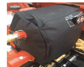
Radiant Lined Black Poly is used to insulate mud pumps.
