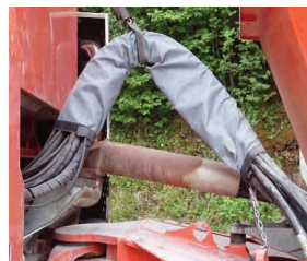
TGS covers & protects hoses from exhaust pipe on mining truck.
