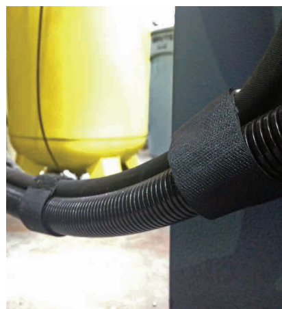
Vibratory hoses in manufacturing environments use Grip Straps to bundle expensive electrical lines.
