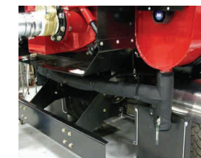
Use Radiant Lined Black Poly to insulate critical lines on Vac trucks.
