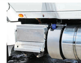
Diesel Exhaust Fluid (DEF) tanks are insulated with Radiant Lined 1050.
