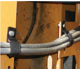
Hanging Straps provide a documented part location & allow access without the need for tools.
